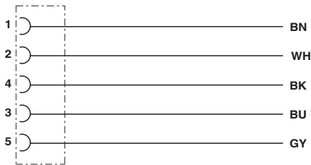
Contact assignment of the M12 socket
