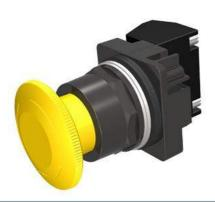
30mm BlackMax, Epoxy Coated Corrosion Resistant Complete Metal Unit Twist-to-Release Operator Non-Illuminated Mushroom Head Cap Small 1.79" (45 mm) Plastic Cap, Yellow 2 Position Maintained, Twist-to-Release with 1 N.O. - 1 N.C. Heavy Duty Contacts, A600/P600 UL Listed, CSA Certified NEMA 1,3,3R,4,4X,12,13 & Automotive Standards
