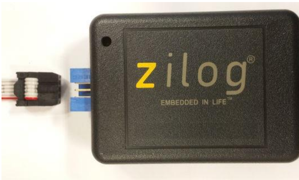
Figure 2. Connecting the 6-Circuit Ribbon Cable to the Encore! SmartCable
