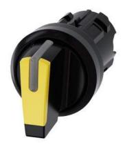
Selector switch, illuminable, 22 mm, round, plastic, yellow, selector switch, short, 3 switch positions I-O<II, left latching, right momentary contact type, actuating angle  $2x45^{\circ}$ , 10:30h/12h/13:30h, with laser labeling, lower case
