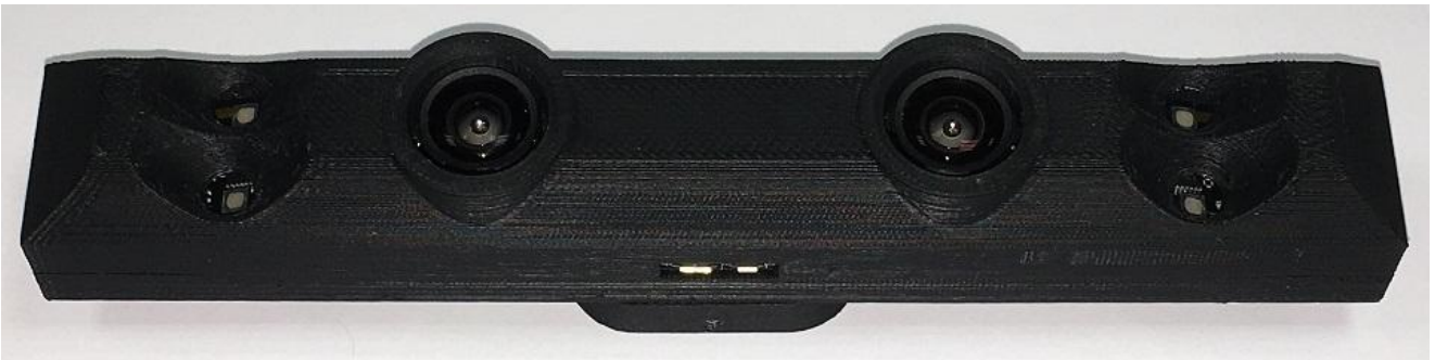
Figure 2. eAP87606A01 6cm baseline with IR illumination
