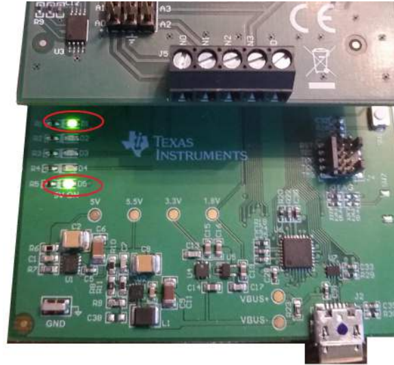
Figure 2-4. LED Indicators D1 and D5
