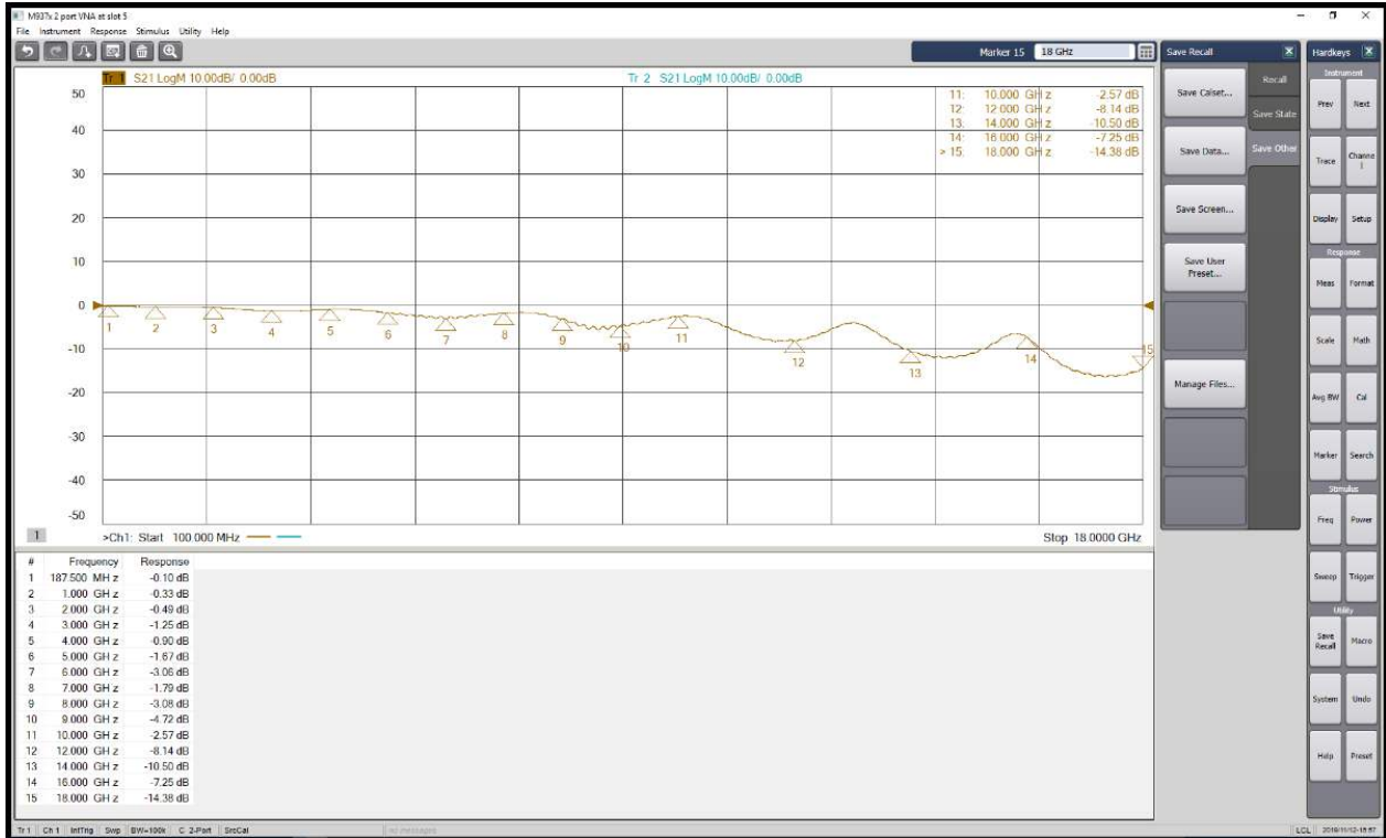
Figure 14. 8V97003 EVB Revision C Transmission Line Loss
