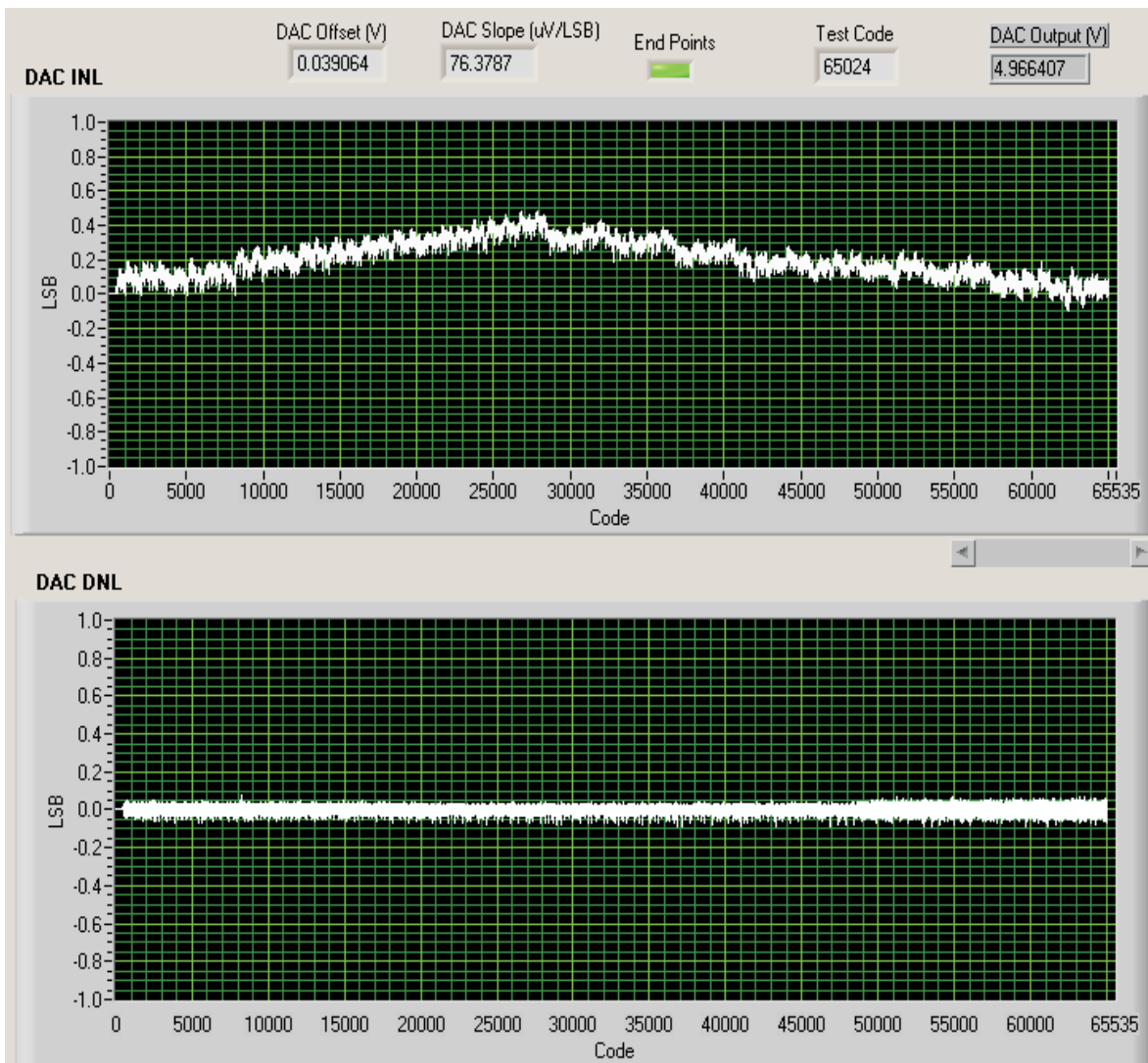
Figure 9. INL and DNL Characteristic Plots
