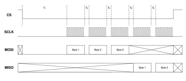
$t_1 = SPI Delay Time to Initial SCLK$
