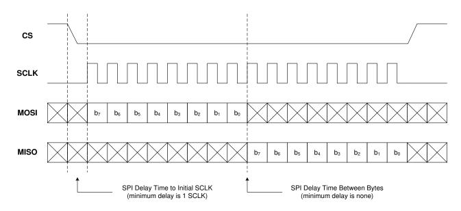
**SPI Master Example #2:** A single byte command is sent to the SPI Slave while a two byte response from the SPI Slave occurs using full-duplex communication. The Delay Time to Initial SCLK is set to 1 SCLK and the Delay Time Between Bytes is set to none or no delay.
