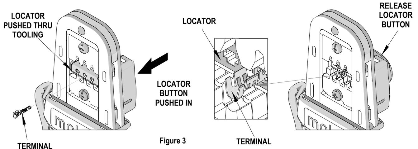
3. While holding the locator button in, load the terminal into the proper nest opening in the locator based on the wire gauge or terminal type markings on the hand tooling. See Figure 3.
