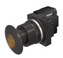
30mm BlackMax, Epoxy Coated Corrosion Resistant Complete Metal Unit Illuminated Push-Pull Operator Transformer type, 120V AC Incandescent Lamp Mushroom Head Cap Small 1 3/4" (44.5 mm) Metal, Black with Amber Lens 2 Position Maintained, Pull-to-Release UL Listed, CSA Certified NEMA 1,3,3R,4,4X,12,13 & Automotive Standards
