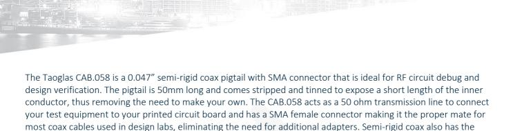
In order to make a proper connection to the PCB without causing an impedance mismatch, the cable jacket needs to be soldered to the PCB ground and the inner conductor gets soldered to the RF transmission line. The CAB.058 has a smooth, semi-rigid, metallic jacket that makes it very easy to solder the jacket to the PCB ground.
