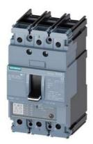
circuit breaker 3VA5 UL frame 125 3-pole, starter protection TM120M, AM, In=50A without overload protection short-circuit protection li=5...12 x In cable connection on both sides
