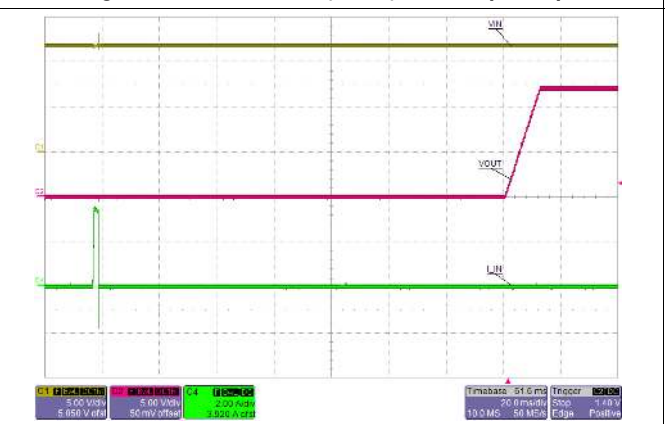
TPS25926x, V_{VIN} = 12\text{ V} , C_{dVdT} = 1\text{ nF}
