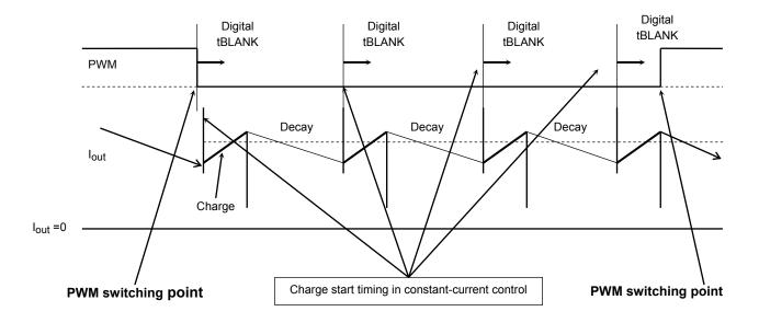
The digital tBLANK time is inserted immediately after the switching timing of externally applied PWM signals, CLK\_X, ENABLE\_X (such as the switching timing between short brake and charging), and also when the charging in constant-current chopper drive is started.
