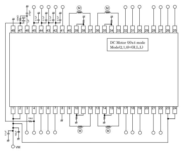
Note: It is recommended that a bypass capacitor is added if necessary. The GND wiring must become one-point-earth as much as possible.
