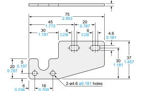
Material: Cold rolled carbon steel (SPCC) (Uni-chrome plated)
