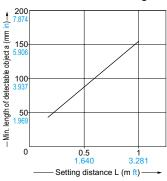
The minimum length of the detectable object, which lies in a plane perpendicular to the sensor front surface, varies with the setting distance, as shown in the left graph. However, note that the minimum length of the detectable object also varies with the object thickness.
