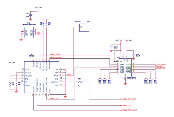
The attached schematic is an example of the ISM420R1 being connected to a 3.3v microcontroller. The output on the ISM420R1 is 1.8 Volts only so a translator chip was used in this design. Please note:
