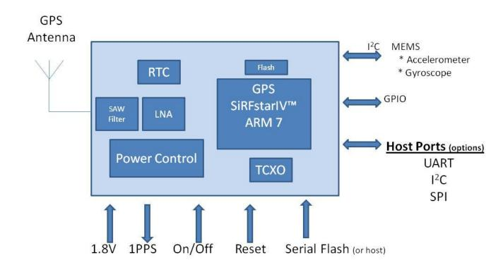
Figure 1 Inventek's ISM420R1-CX General Block Diagram
