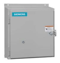
Non-reversing NEMA contactor, Size 2, Three phase full voltage, Contactor amp rating 45A, 3 wire (NO aux included), 110-120/220-240VAC 60Hz coil, Noncombination type, Encl. NEMA type 4X fiberglass, Water/dust tight noncorrosive, Standard width enclosure
