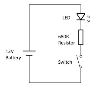
The circuit diagram for the torch is shown above. It is a very simple circuit, powered by a 12 Volt battery.
