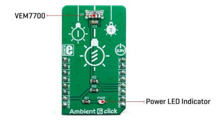
The VEML7700 sensor uses only six 16-bit registers, which makes it very simple to configure and use. Even though, it comes with the mikroSDK compatible library, which simplifies the development even more. However, more detailed explanation of each command can be found in the datasheet of the VEML7700, if required.
