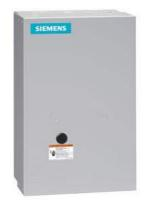
Electrically held lighting contactor, Contactor amp rating 30A, 0 N.C. / 9 N.O. Poles, 480VAC 60HZ coil, Non-combination type, (no disconnect device), Enclosure NEMA type 1, Indoor general purpose use
