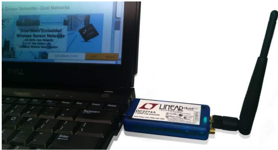
Figure 8 SmartMesh IP USB Manager (DC2274A-A) in PC
