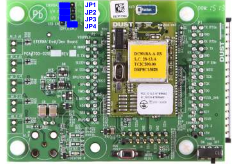
Figure 4 DC9018A-B and DC9018A-A 4 Board Jumpers
