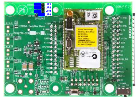
Figure 5 DC9018B-B and DC9018B-A 5 Board Jumpers
