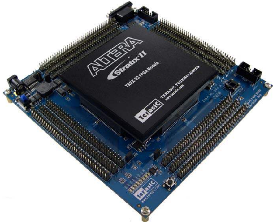
Figure 1.2. TRES-S2 FPGA module plugged onto the TRES-S2-TMA motherboard
