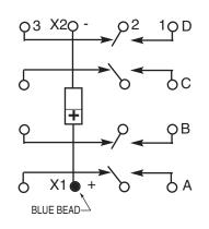
**NOTE:** Polarity must be observed with DC coil supply. Relay is polarized with a permanent magnet and will not operate or be damaged by reverse polarity.
