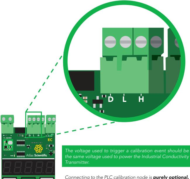
Connecting to the PLC calibration node is **purely optional**. Leaving it disconnected will have no effect on the Industrial Conductivity Transmitter's operation.
