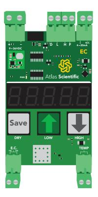
The first option is "ProbE". Press the green LOW (up) or gray HIGH (down) buttons to select you probe type. Press the gray DRY (save) button when the correct probe type has been selected. The probe type selection is now complete.
