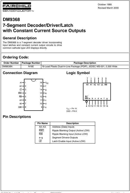
DM9368 7-Segment Decoder/Driver/Latch with Constant Current Source Outputs
