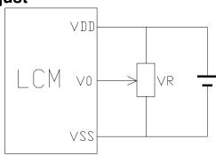
VDD~V0: LCD Driving voltage
