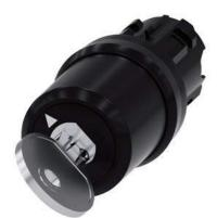
Key-operated switch BKS, 22 mm, round, plastic, Lock No. E7 (VW), without key, 2 switch positions O-I, latching, actuating angle 90°, 10:30h/13:30h, key removal O+I, with laser labeling, inscription or symbol Customer-specific selection with SIRIUS ACT configurator (CIN)
