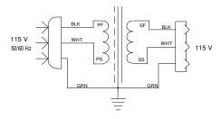
$<sup>^{\</sup>star}$  Leakage current between primary and secondary is typically measured at less than 10  $\mu A.$
