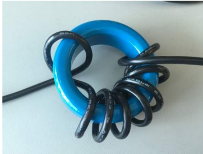
Figure 17. USB Cable Around Ferrite Bead
