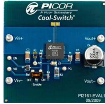
Figure 1: PI2161-EVAL1 Evaluation Board (1.8" x 1.8")
