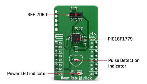
This Heart Rate 9 Click board™ introduces Microchip's proprietary method (hereafter "proprietary method") of measuring multiple signals in a body using pseudorandom binary sequence generation and phase division multiplexing. This proprietary method uses a special encoding/decoding scheme to allow multiple light-emitting diodes (LED) transmitting light simultaneously with a single photodiode to condition each light from the combined lights at the receiving side.
