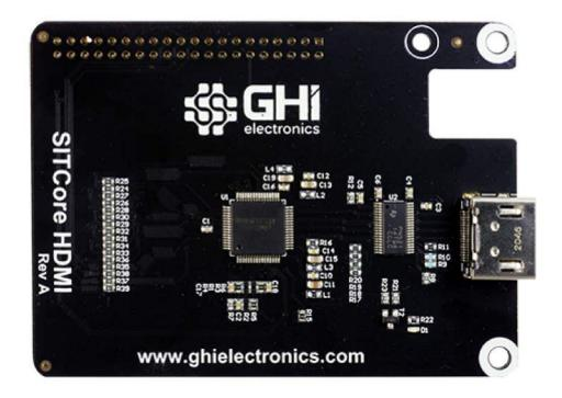
This optional HDMI adaptor can be used instead of the display to provide an HDMI option. The board utilizes TI's TFP410 HDMI transmitter chip.
