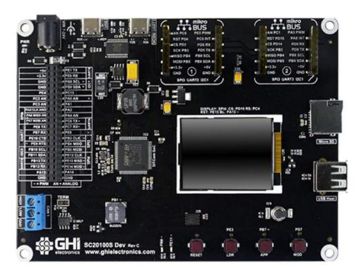
The SC20100S Dev Board includes an SC20100S soldered to the board and a built in 1.8 inch color serial display. It has a 40 pin socket headers for connecting peripherals. Peripheral connectors include two mikroBus connectors, external power, CAN, USB host and client, RTC supercap and an SD card slot. It also has a buzzer, LEDs, a reset button, and user programmable boot buttons.
