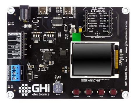
The SC13048Q Dev Board includes an SC13048Q soldered to the board and a built in 1.8 inch color serial display. It has a 10 pin socket header for connecting peripherals. Peripheral connectors include mikroBus connector, external power, CAN, USB host and client and RTC backup supercap. It also has a buzzer, LEDs, a reset button, and user programmable boot buttons.
