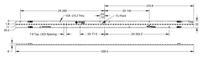
1. Four Poke-In Connectors accept 18-24 AWG solid or stranded wire
