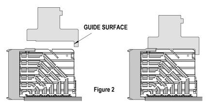
Using the application tool and an appropriate press, seat the Daughtercard module until there is less than 0.10mm (.004 in) clearance between the bottom of the plastic housing and the surface of the PCB. See Figure 3.
