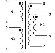
N2 denotes two windings connected in parallel. Terminals 5+6 and 7+8 must be tied as solder
