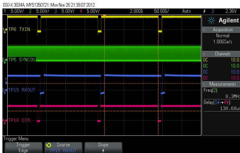
Figure 10. System Evaluation with U1 as Transmitter and U2 as Receiver at 115.2kbps
