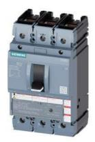
circuit breaker 3VA5 UL frame 250 breaking capacity class M 35kA @ 480 V 3-pole, line protection TM230, FTAM, In=90A overload protection Ir=90A fixed short-circuit protection Ii=5...10 x In UL489 SB (naval), 50 deg. cel. cable connection on both sides
