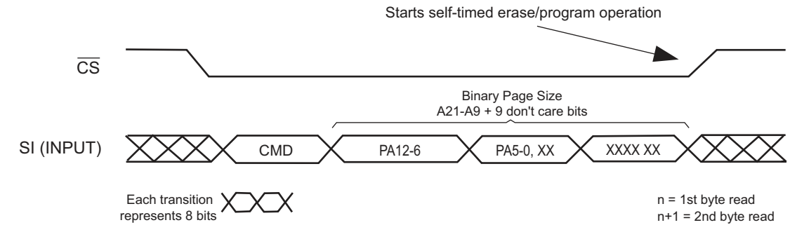
Figure 20-3. Buffer to Main Memory Page Program (Data from Buffer Programmed into Flash Page)
