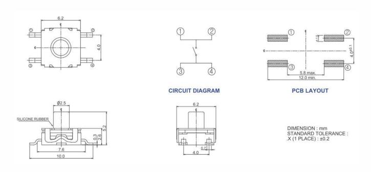
Figure 2 – 222KJA, Surface Mount J-Bend Terminal, Actuator Height 5.2mm
