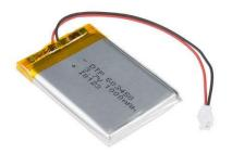
**Description:** These are very slim, extremely light weight batteries based on Lithium Ion chemistry. Each cell outputs a nominal 3.7V at 1000mAh! Comes terminated with a standard 2-pin JST-PH connector - 2mm spacing between pins. These batteries require special charging. Do not attempt to charge these with anything but a specialized Lithium Polymer charger.
