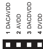
Figure 3–6. Jumper Block J3 on the DAC1220EVM
