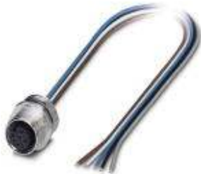
Sensor/Actuator flush-type socket, 5-pos., M12, A-coded, front/screw mounting with Pg9 thread, with 0.5 m TPE litz wire, 5x 0.34 mm 2
