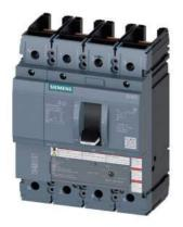
circuit breaker 3VA5 UL frame 250 breaking capacity class C 100kA @ 480V 4-pole, line protection TM210, FTFM, In=80A overload protection Ir=80A fixed short-circuit protection Ii=10 x In N conductor unprotected without connection
