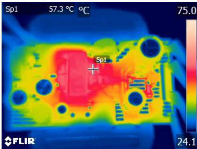
Figure 20 – Transformer Side. 265 VAC, Full Load.
