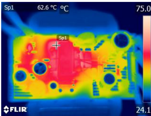
Figure 18 – Transformer Side. 90 VAC, Full Load.
