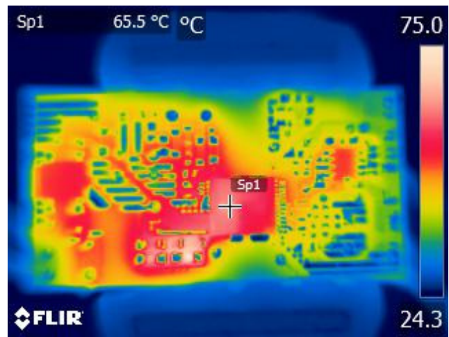
Figure 19 – InnoSwitch3-EP Side. 90 VAC, Full Load.
