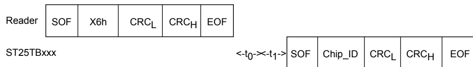
Figure 49. Slot_marker frame exchange between reader and ST25TB04K
