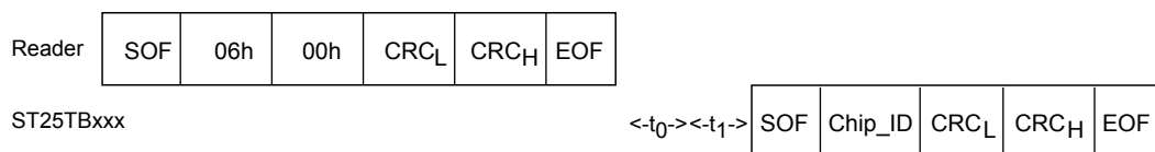
Figure 20. Initiate frame exchange between reader and ST25TB04K
