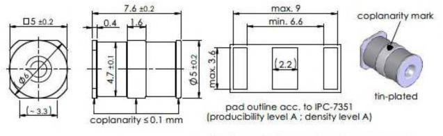
\* for reflow soldering, coplanarity mark upwards
