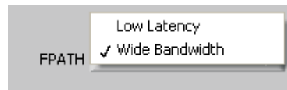
Figure 11. Low-Latency or Wide-Bandwidth Digital Filter
