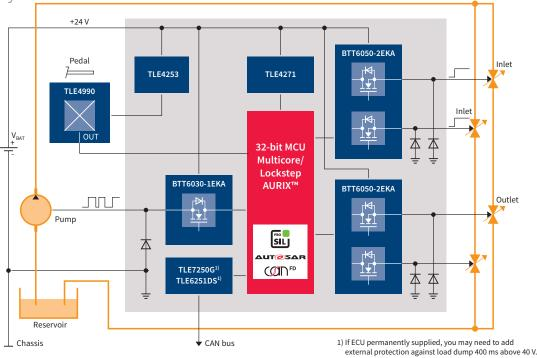
Hydraulic management system has to be precise and robust enough to withstand harsh environments and engineered to carry out a variety of protective and diagnostic functions.
