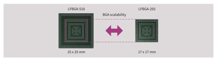
> LFBGA-292 and LFBGA-516 are ball compatible so that customers can build one PCB for both packages
