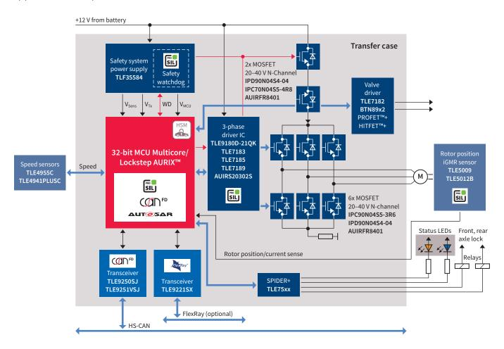
In Four-Wheel Drive (4WD) and All-Wheel Drive (AWD) vehicles, the transfer case is the part of the drivetrain responsible for the transfer of torque from the transmission to the front and rear wheels. The market now demands increased performance to drive BLDC motors and ever-greater functional safety requirements. AURIX™ has the state-of-the-art safety features required to enable systems to achieve ASIL-D, the highest safety level.
