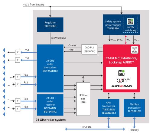
The new TriCore™ AURIX™ family will enhance classic safety features with dedicated features to meet the needs of 24 GHz radar systems. The combination of new features and increased SRAM, in conjunction with outstanding safety features, enables a high level of integration and reduction of complexity.
