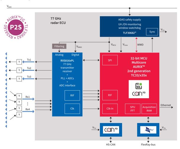
Thanks to its proprietary radar accelerator IP, the new TriCore™ AURIX™ TC3xx family will bring another level of performance to radar applications, as well as fulfilling the ever-growing requirements regarding safety and security in the ADAS market.
