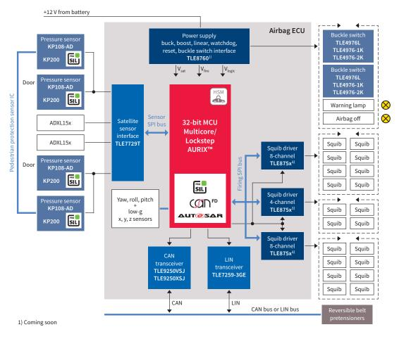
Thanks to its state-of-the-art safety features, the new TriCore™ AURIX™ family enables systems to achieve the highest safety level up to ASIL-D. Its scalability allows the selection of a single-core solution for basic airbag systems and multicore solutions for airbag systems with an integrated sensor cluster. The best cost-performance fit is offered by the wide range of flash, performance and peripheral options available within the AURIX™ family.
