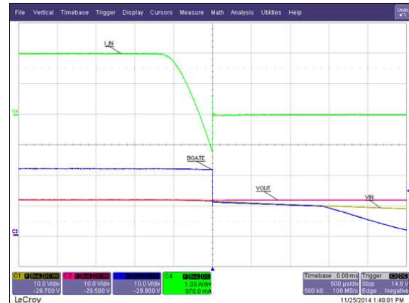
Figure 14. Gradual Reverse Current
