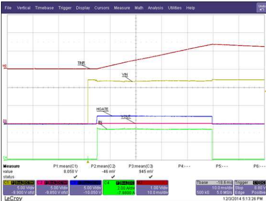
Figure 11. Start into Short on VOUT
