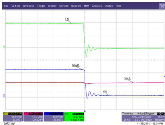
Figure 13. Hot – Short on VIN
